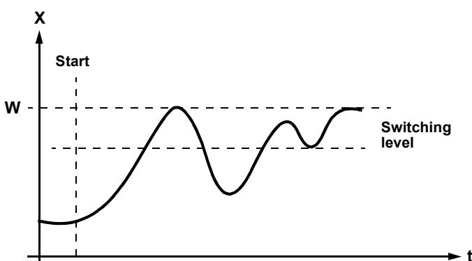
If there is a **large difference between actual value and setpoint** when "tunE" is activated, a switching line is established around which the controlled variable performs forced oscillations during the self-tuning procedure. The switching line is set at such a level that the actual value should not exceed the setpoint.
